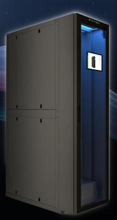
CITEC Rack Cooling series is a pre-assembled, self-contained integrated solution with key Data Center equipment's installed within a compact rack unit which includes precision cooling unit, power management unit, environment monitoring system, UPS and power distribution unit that cater for Edge applications.
